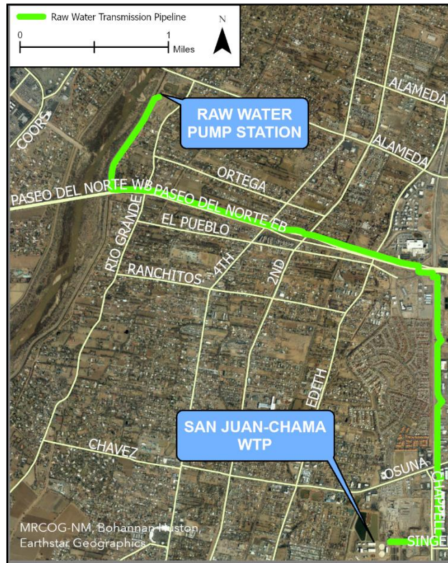
Figure 5-5: Raw Water Transmission Pipeline Route
